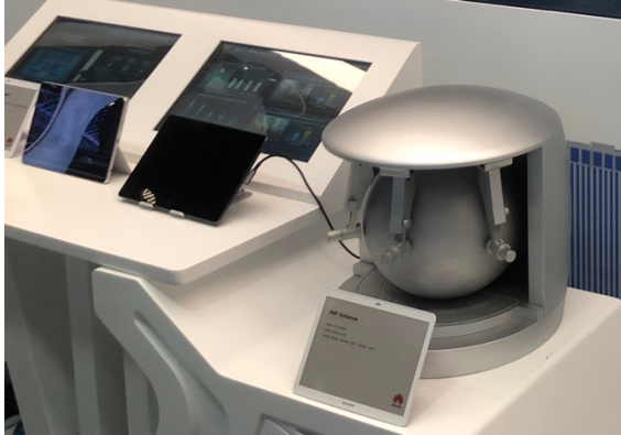
Figure 13 Huawei's spherical lens antenna is equivalent to 8 microwave parabolic antennas—one of the show's highlights hidden behind the company's security cauldron!
