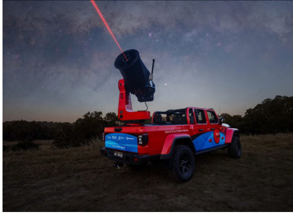
Figure 4 TeraNet TN-3 mobile OGS. [Source: TeraNet]
